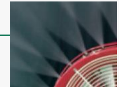
Yamabiko nozzle during spraying (fan shape) (average particle diameter 110~270 microns)
